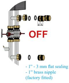
**Attention** – the shorter part of the thread of the nipple is intended for screwing into the swivelnut.
