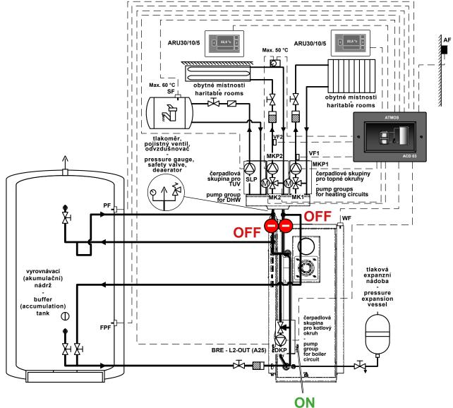
The operation of the boiler fan is controlled from the ATMOS A25 pellet burner.
