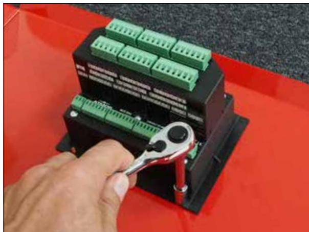
Attention - do not overtighten (right-hand thread)
