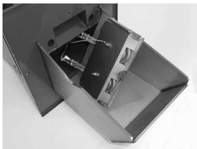
Fig. 4 - Disassembled plate with the ignition spirals
