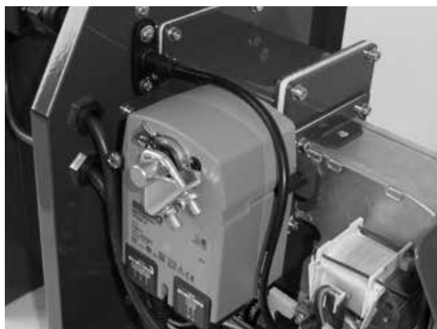
Fig. 11 - special servo controlled flap
