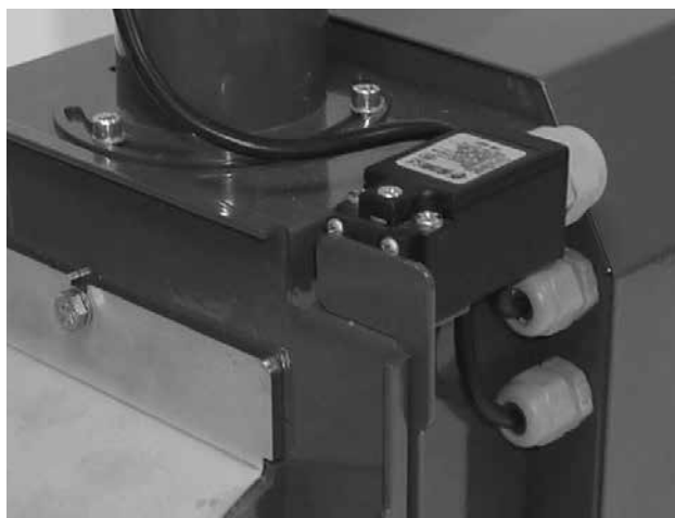
Fig. 8 - End switch with a special stop
