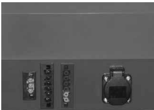
Fig. 12 - Burner with two 6-pin connectors, left - power, right - sensors, 3-pin connector for connecting speed sensor of the boiler's fan and socket for conveyor
