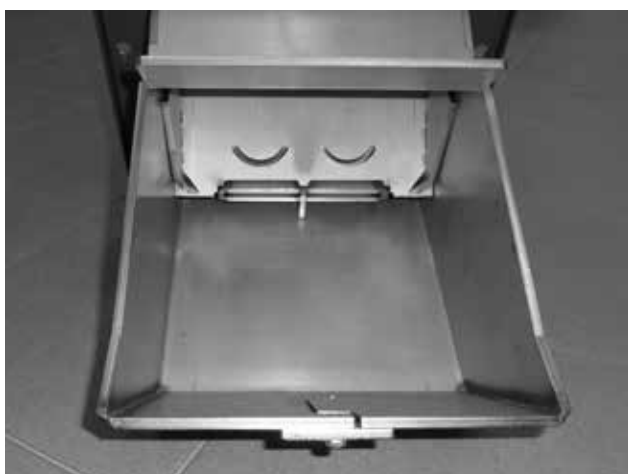
Fig. 3 - Combustion chamber with the nozzle of the pneumatic cleaning and opening for 2 ignition spirals
