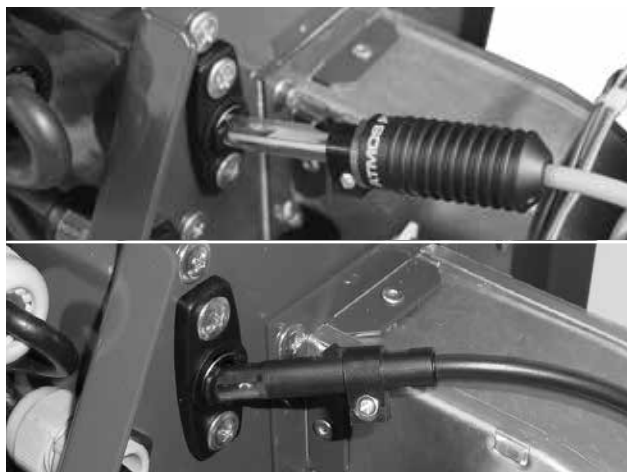
Fig. 6 - Photocell - be careful about its proper orientation - we recommend you to clean it at least once a year new fotocell / old fotocell
