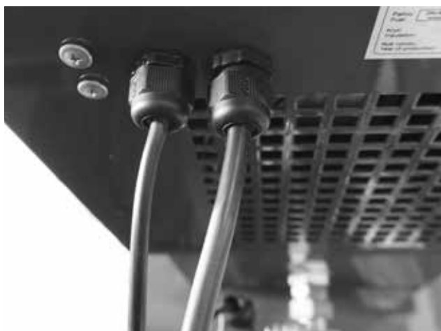
Fig. 11 - connection of electric valve and comperssor for pellet burner pneumatic ash cleaning system
