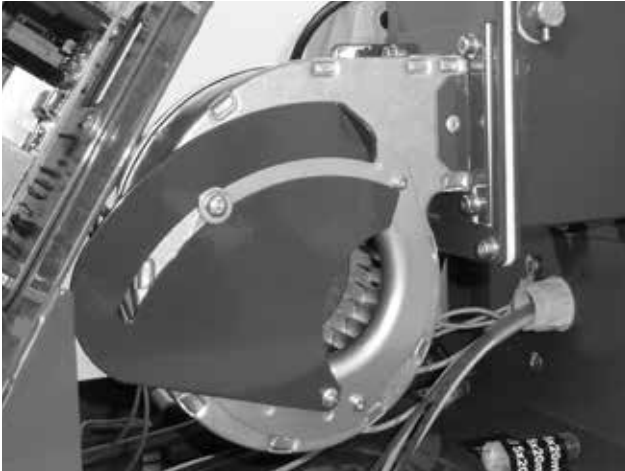
Fig. 7 - Burner fan with an air flap
