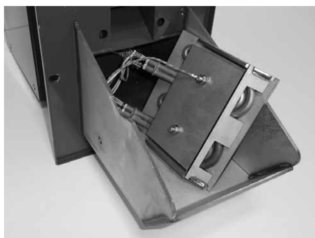
Fig. 4 - Disassembled plate with the ignition spirals
