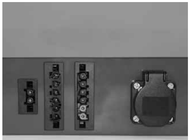
Fig. 12 - burner – two 6-pin connectors: left for power, right for sensors, a 2-pin connector for additional cable (R3 and R4) and a socket for conveyor
