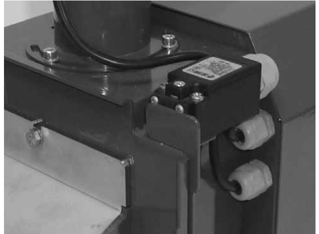
Fig. 8 - End switch with a special stop
