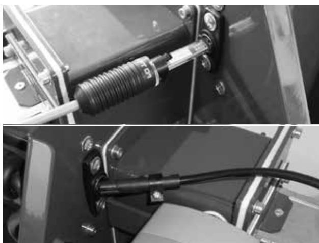
Fig. 6 - Photocell - be careful about its proper orientation - we recommend you to clean it at least once a year new fotocell / old fotocell
