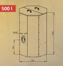
The **middle sized** silo is suitable for all boilers designed for smaller boiler rooms where larger silos cannot be used. It contains 325 kg of pellets which means approximately 1463 kWh (21 bags).
