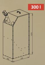
AZPD 300 – a set of 300 l silos with DRA25 conveyors – 1,3 m which is suitable for small boiler rooms. It can be placed beside the boiler to fit into smaller spaces. The 300 litre silo contains 195 kg of pellets which provides about 880 kWh (13 bags).
