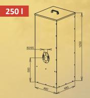
The **smallest** silo is suitable for all boilers designed for smaller boiler rooms where larger silos cannot be used. It contains 163 kg of pellets which means approximately 730 kWh (10 bags).
