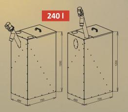
**AZPD/AZPU 240** – a set of 240 l silos with DRA25 conveyors – 1,3/1,7 m which is suitable for small boiler rooms. It can be placed beside the boiler to fit into smaller spaces. The 240 litre silo contains 156 kg of pellets which provides about 700 kWh (10 bags).
