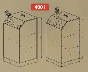
AZPD/AZPU 400 – a set of 400 l silos with DRA25 conveyors – 1,3 m which is suitable for small boiler rooms. it can be placed beside the boiler to fit into smaller spaces. The 400 litre silo contains 260 kg of pellets which provides about 1170 kWh (17 bags).
