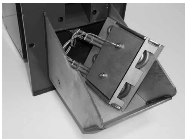
Fig. 4 - Disassembled plate with the ignition spirals
