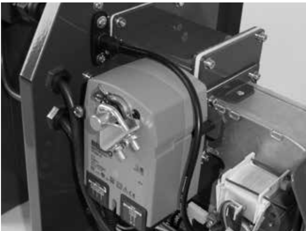
Fig. 11 - special servo controlled flap
