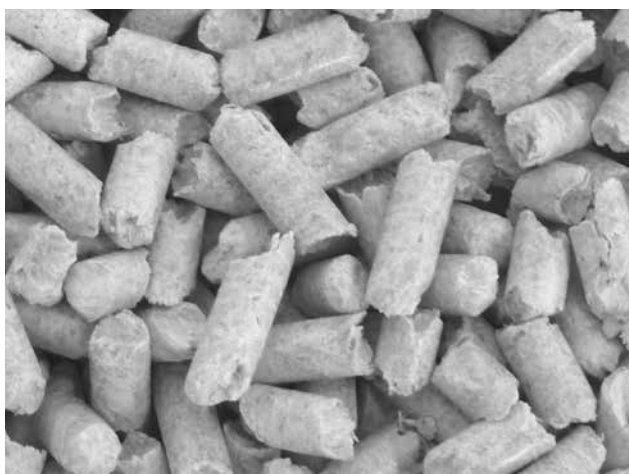
Fig. 17 – High-quality wooden pellets – white without black dots (bark)
