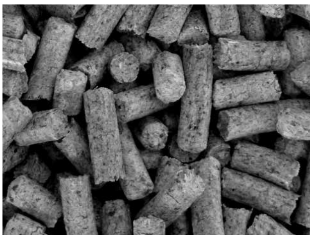
Fig. 18 – Poor-quality wooden pellets – dark with bark (with black dots)
