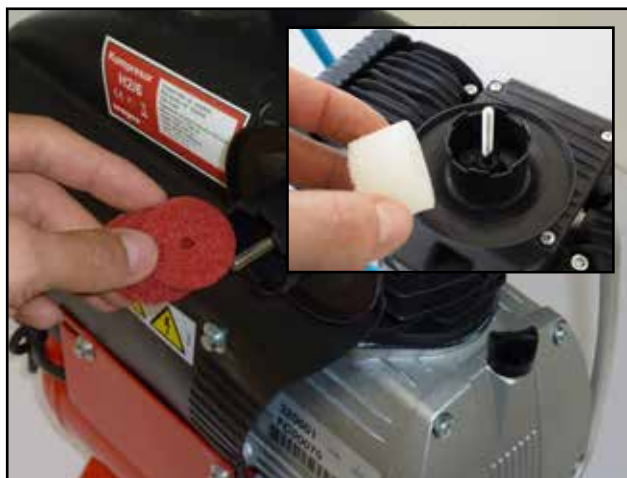
Cleaning compressor filter
