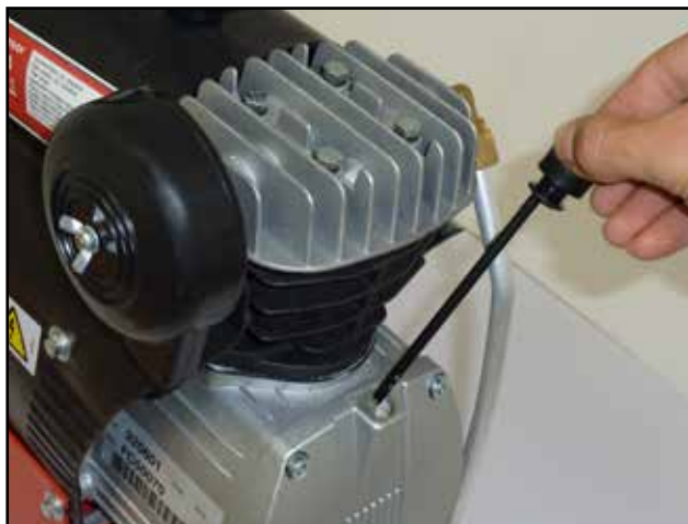
Checking oil levels in compressor
