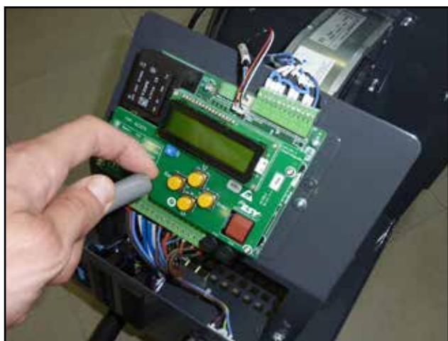
Example of cleaning (blow out) space inside the burner. (without power!)
