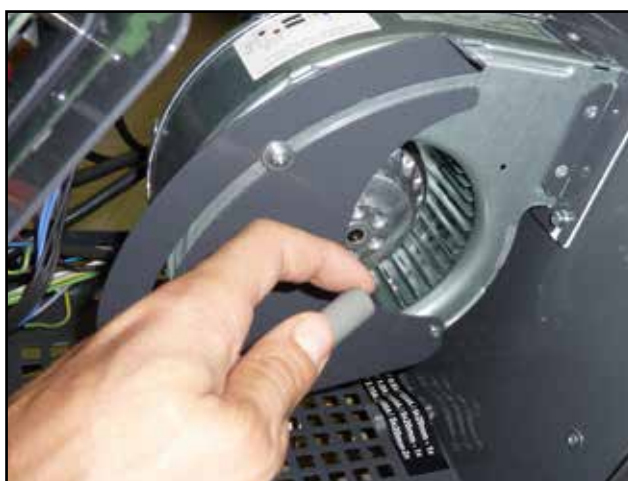
Example of cleaning (blow out) pressure fan impeller of the burner once a season
