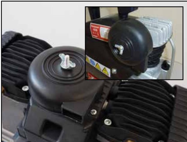
Photo of suction filter screwed onto compressor
