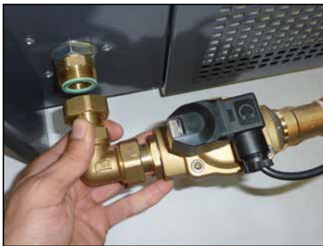
Take complete screw fitting with solenoid control and connecting cable and screw it to the burner
