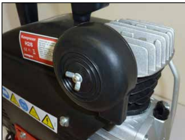
Photo of suction filter screwed onto compressor
