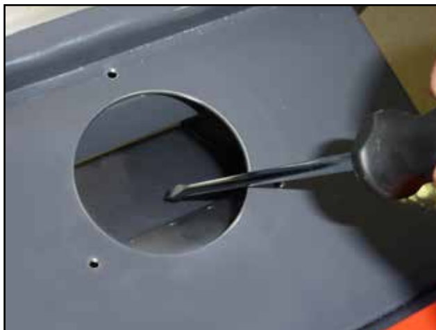
Example of cleaning the space under the pellet inlet tube
