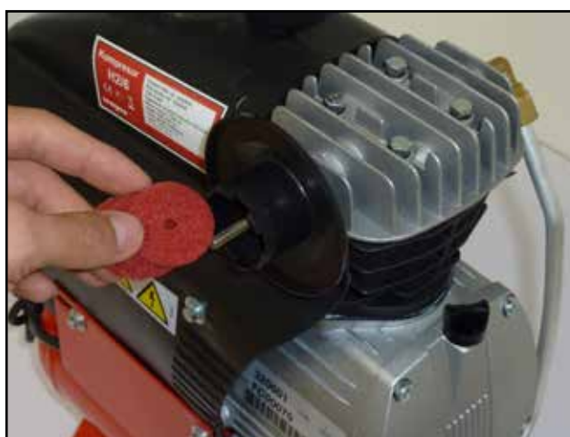
Cleaning compressor filter
