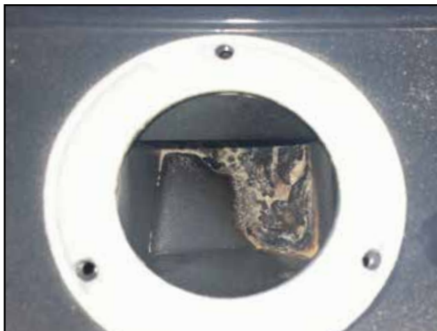
Clogging after 3 months use with crushed pellets with large amount of dust
