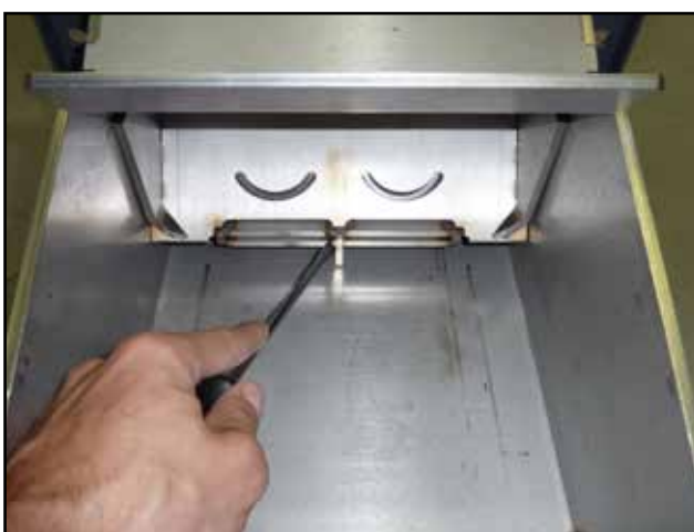
Example of cleaning the front part of the compressed air inflow channel
